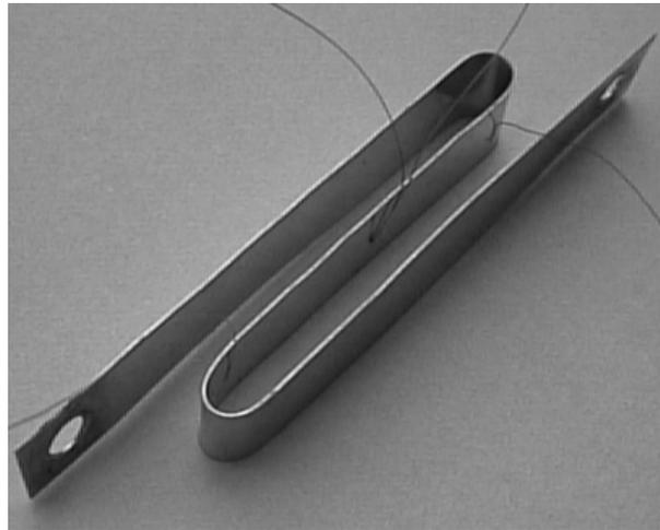
**Fig. 3.** Sample with thermocouple and voltage probes.
