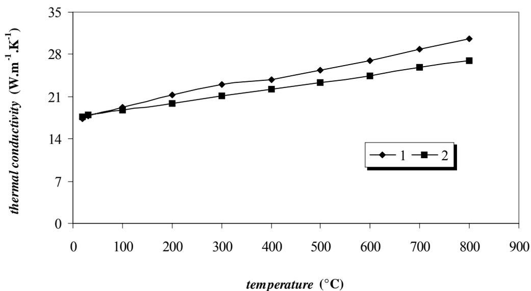
**Fig. 6.** Dependence of thermal conductivity on temperature.
