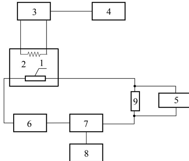
**Fig. 1.** Block diagram of experimental apparatus. 1 – sample, 2 – furnace, 3 – programmable power supply, 4 – controller, 5 – data logger, 6 – battery, 7 – power switch, 8 – timer, 9 – standard shunt.
