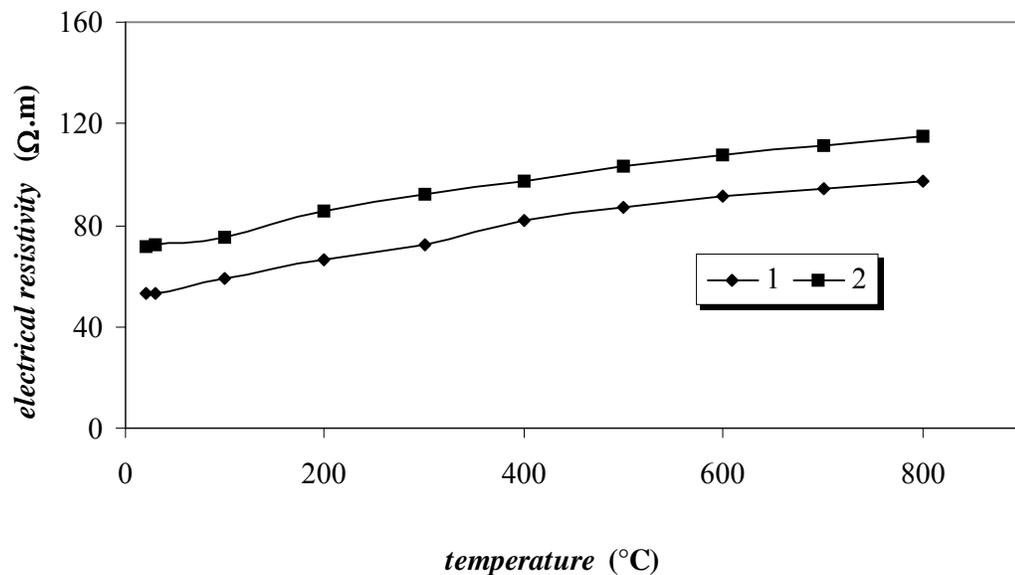
**Fig. 5.** Dependence of electrical resistivity on temperature.
