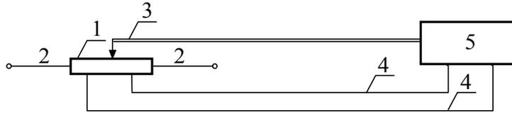
**Fig. 2.** Detail of temperature and voltage sensing. 1 – sample, 2 – electric energy supply leads, 3 – thermocouple, 4 – voltage probes, 5 – data logger.
