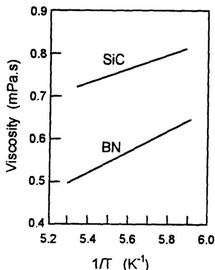
Figure 1 Viscosity of Si as measured in wetting SiC and non-wetting BN crucibles<sup>1)</sup>.
