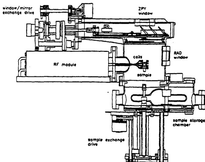
Figure 2 Schematic diagram of the oscillating drop apparatus used to measure viscosities of molten amorphous metals in microgravity.
