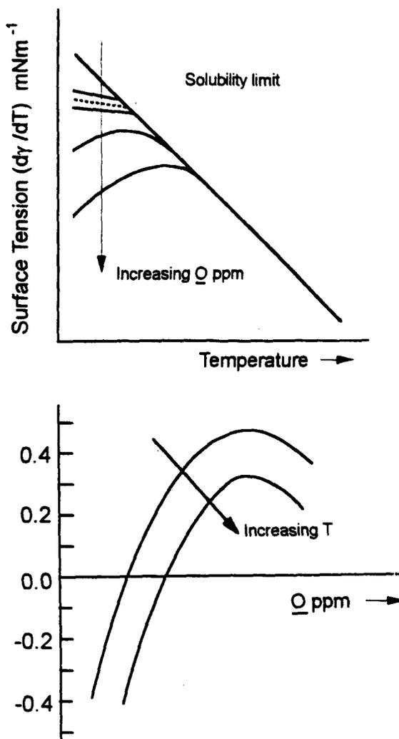
Figure 3 Schematic diagrams showing the effect of (a) both  $\underline{O}$  content and temperature on surface tension; - - - denotes saturation limit of O in metal and (b) on the temperature coefficient.
