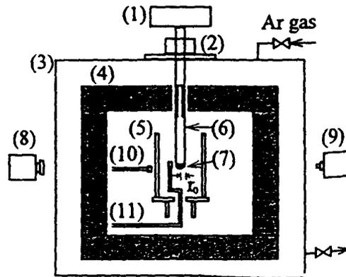
Figure 4 Schematic diagram showing the dynamic hanging drop apparatus. (i) speed control motor, (2) vacuum shaft, (3) main chamber, (4) insulation, (5) carbon heater, (6) carbon rod, (7) hanging drop, (8) high speed camera, (9) IR thermometer, (10) thermocouples.
