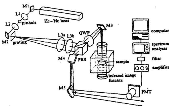
Figure 5 Schematic diagram showing SLLS method.
