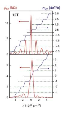
Fig. 8 Resistivity (red) and Hall conductivity (blue) as a function of carrier concentration in graphene (top) and bilayer graphene (bottom). (Reprinted with permission from<sup>15</sup> (top) and from<sup>47</sup> (bottom). © 2005 and 2006 Nature Publishing Group.)
