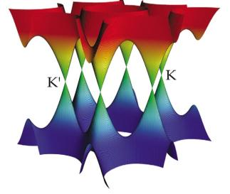
Fig. 3 Band structure of graphene. The conductance band touches the valence band at the K and K' points.
