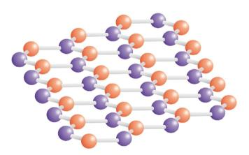
Fig. 4 Crystallographic structure of graphene. Atoms from different sublattices (A and B) are marked by different colors.
