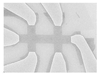
Fig. 5 Scanning electron micrograph of a graphene device. The graphene crystal is contacted by Au electrodes and patterned into Hall bar geometry by e-beam lithography with subsequent reactive plasma etching. The width of the channel is 1  $\mu$ m. (Courtesy of K. Novoselov and A. Geim.)
