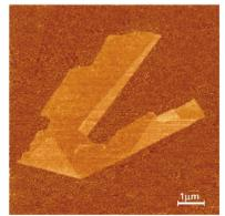
Fig. 2 Atomic force microscopy image of a graphene crystal on top of an oxidized Si substrate. Folding of the flake can be seen. The measured thickness of graphene corresponds to the interlayer distance in graphite. Scale bar = 1  $\mu$ m. (Reprinted with permission from<sup>13</sup>. © 2005 National Academy of Sciences.)
