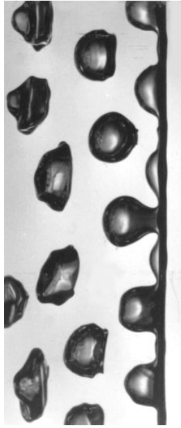
d. Film boiling of acetone on a 22 gage wire at earth-normal gravity. The true width of this image is 3.48 cm.
