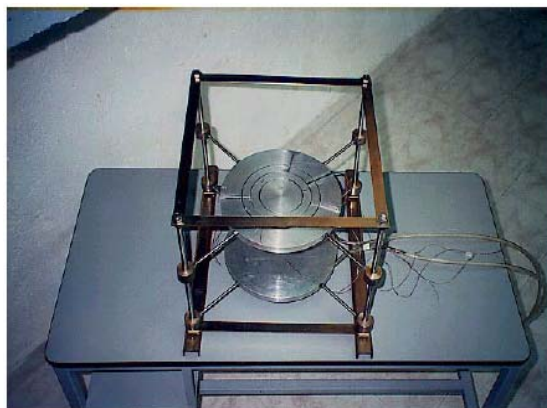
Figure 1: Guarded hot-plate apparatus for measuring thermal conductivity of insulating solid materials.
